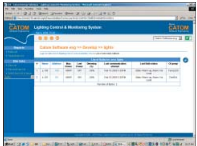
List of Area Faulty Ballasts/Bulbs
